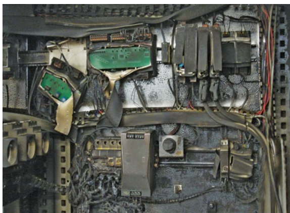
Electronic components damaged by overvoltage
