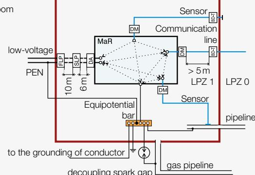
Fig. 2 Coupling between input and output line and earth connection
