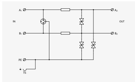
2-core line with one pole connected to common ground.
