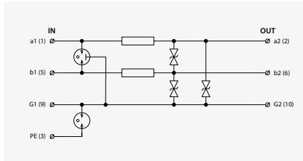
2-3 core line incoming from LPZ 0 to structure with one-pole connected with ground.
