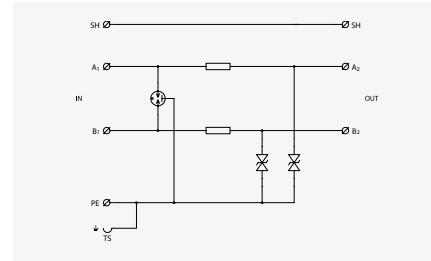
Two single-core lines with common ground.
