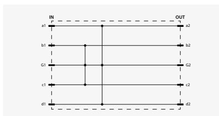
Short-circuiting module for maintenance of signalling lines.
