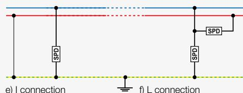
The DC side of the PV system can either be unearthed (insulated) or with one pole earthed. Figures 1 and 2 (see CLC/TS 50539-12) show how SPDs on the DC side must be connected.
