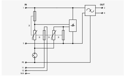
Power supply 24 V up to 6 A with integrated RFI filter.
