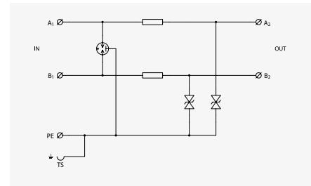
Two single-core lines with common ground.
