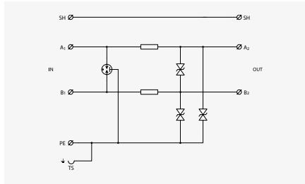
2/3-core line with one pole connected to common ground.
