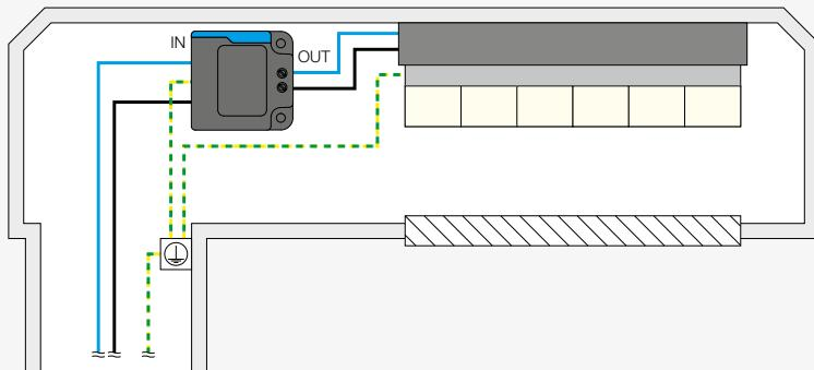
Fig. 02 Wiring of SPD to Class II equipment
