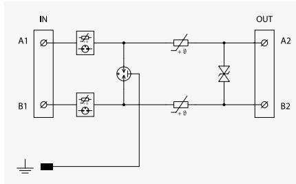
2 core line with current limiting function.
