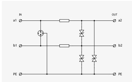
2-3 cores line incoming from LPZ 0 to structure with one-pole connected with ground.
