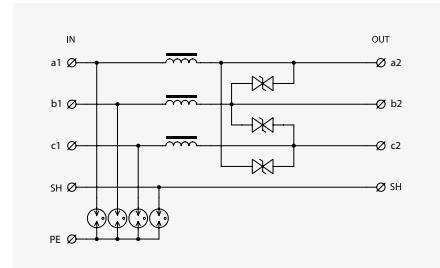
3 core floating line with shielding.
