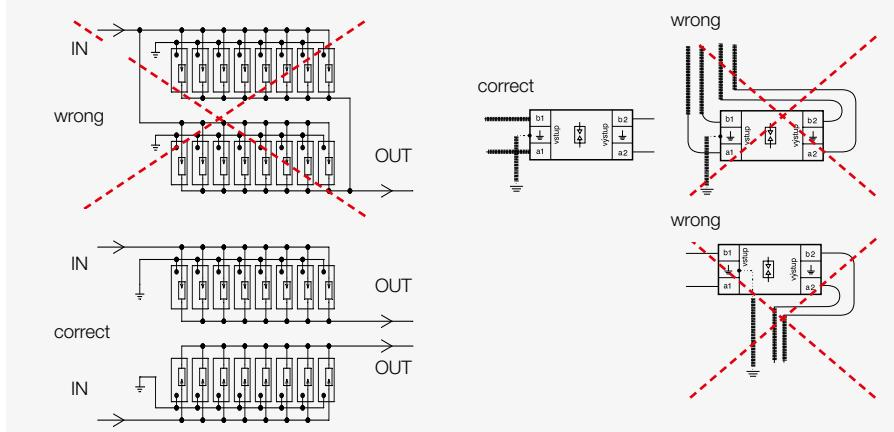
Fig. 3 Principle of the protection of control systems
