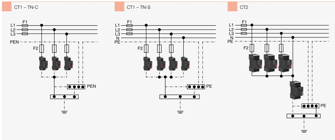
Behind the **FLP-B+C MAXI V...** in low-voltage power network 230/400 V AC is **not required to install any additional SPD** (e.g. SPD type 3) if the **length** of the electrical circuit from the
